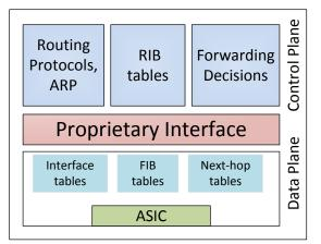
Figure 1. Basic blueprint of an IP router
