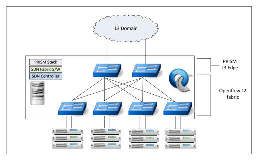
Figure 6. PRISM as L3 edge in Data-Centers
