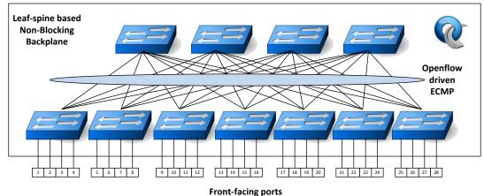
Figure 4. PRISM non-blocking forwarding
