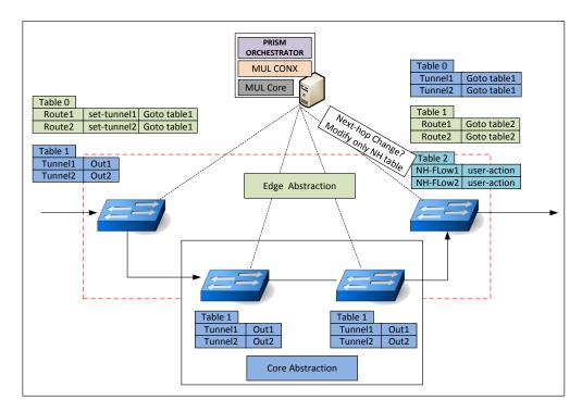
Figure 3. PRISM flow-table optimization
